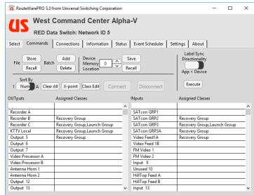
Commands: You can choose an input and output, then pick an action (Connect, Disconnect), or Store and Recall complete or partial configurations from the unit's memory, or your PC. Channel port names can be added, edited or synced
